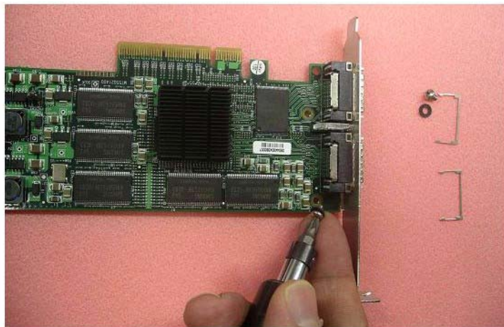
Figure 14: Attach Bracket onto Card using Screws
