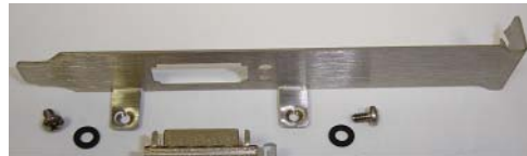
(c) Bracket Separated From Clips and Screws.
